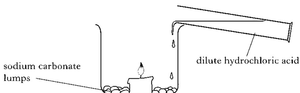
Why would the candle burn for longer if an equal volume and concentration of ethanoic acid was used instead of the dilute hydrochloric acid?
