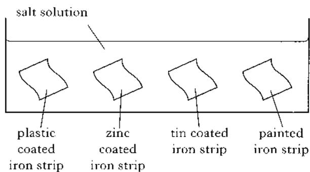
The iron strip which would have rusted most quickly was the one which was
