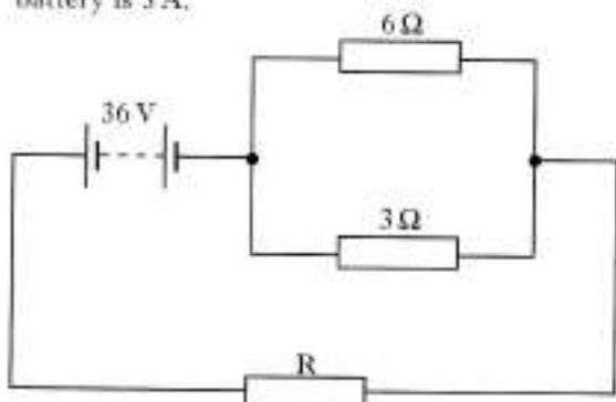
Assuming that the battery has negligible internal resistance, the resistance of resistor R is
