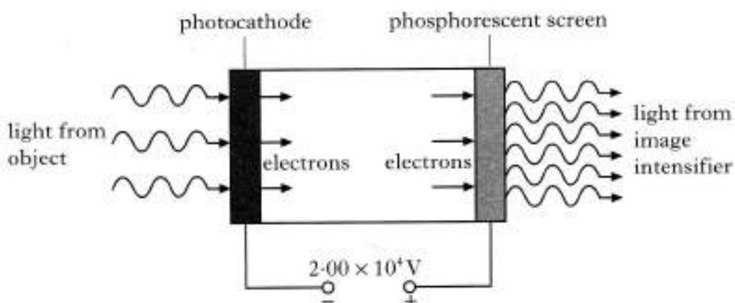
The voltage between the photocathode and the phosphorescent screen is  $2.00 \times 10^4 \text{ V}$ .
