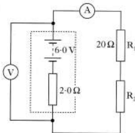
(i) Show by calculation that  $R_2$  has a resistance of 8.0  $\Omega$ .
