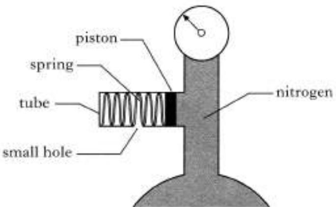
The piston of cross-sectional area  $4.0 \times 10^{-6} \text{ m}^2$  is attached to the spring. The piston is free to move along the tube.
