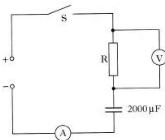
The graphs below show how the potential difference  $V_R$  across the **resistor** and the current  $I$  in the circuit vary with time from the instant switch S is closed.
