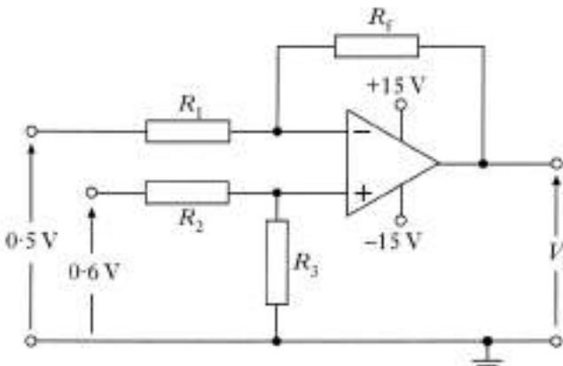
$$R_1 = R_2 \text{ and } R_f = R_3$$
