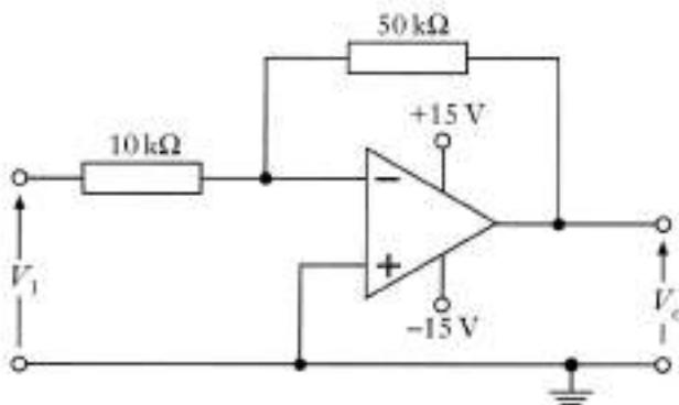
The input voltage  $V_1$  is +5 V. The most likely value for the output voltage  $V_o$  is
