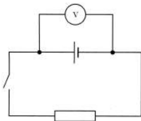
When the switch is open, the student notes that the reading on the voltmeter is 1.5 V. The switch is then closed and the reading falls to 1.3 V.
