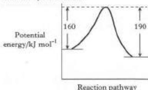
When a catalyst is used the activation energy of the forward reaction is reduced to 35 kJ mol<sup>-1</sup>.
