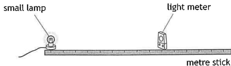
The irradiance of the light from the lamp is measured using the light meter.
