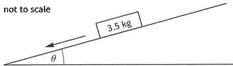
The force of friction acting on the block is 6.4 N.
