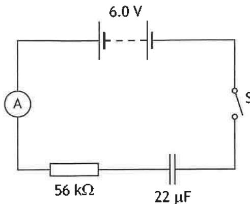
The capacitor is initially uncharged. The student closes the switch and the capacitor takes 6.2 s to fully charge.
