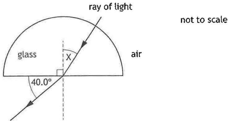
The critical angle for the glass block is  $37.0^\circ$  for this light.
