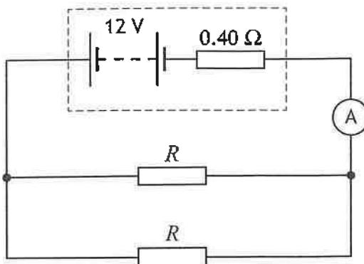
The reading on the ammeter is 4.0 A.
