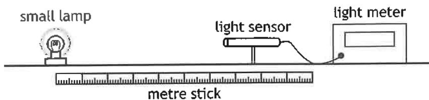
The distance between the lamp and the light sensor is measured with a metre stick.
