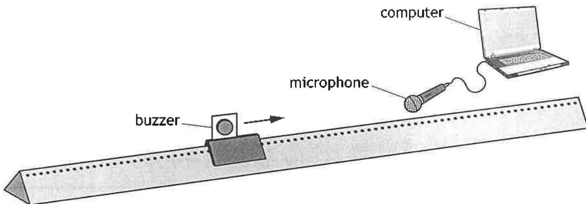
The vehicle is fitted with a buzzer. A microphone is connected to a computer.
