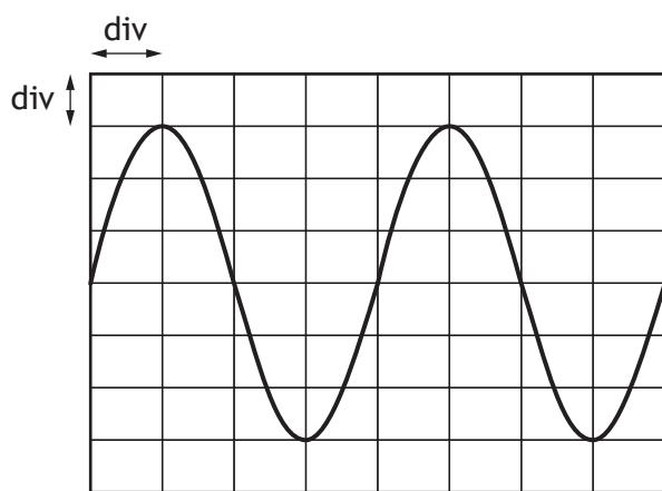
The Y-gain setting on the oscilloscope is 1.0 V/div.
