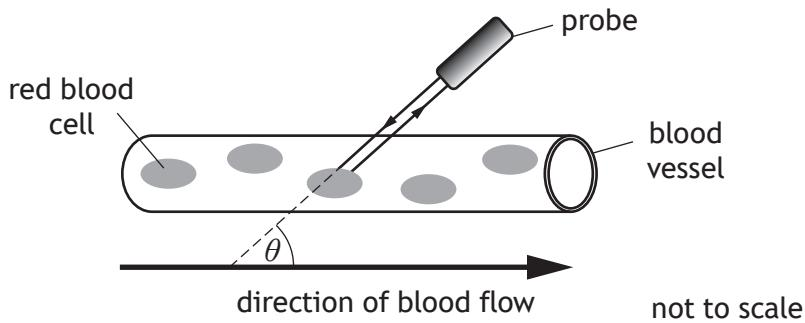
Ultrasound waves are transmitted by a probe. The frequency of the ultrasound waves changes as they reflect from the blood cells. The probe detects the reflected waves.
