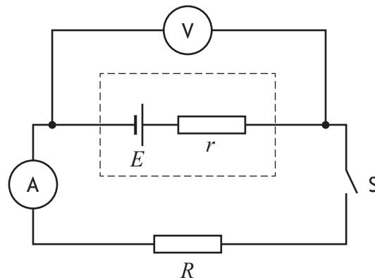
When switch  $S$  is open the reading on the voltmeter is 1.5 V.
