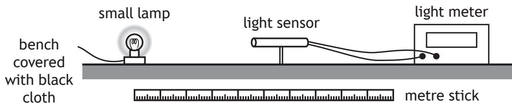
Describe how this apparatus could be used to verify the inverse square law for a point source of light.
