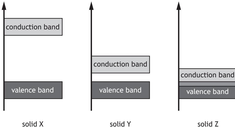
(a) Complete the table to show which solid represents a conductor, an insulator and a semiconductor.
