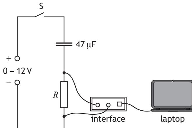
The capacitor is initially uncharged. The switch  $S$  is now closed. A laptop connected to an interface displays a graph of current against time as the capacitor charges.
