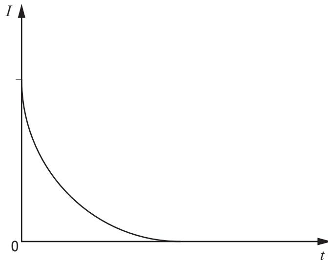
Switch S is opened, and the capacitor is discharged.
