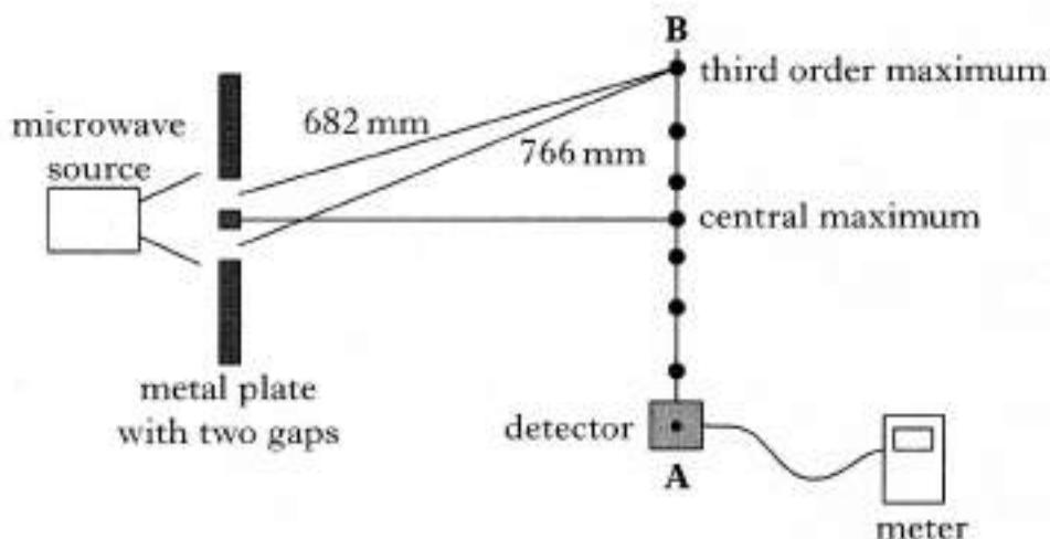
(i) As the detector is moved from **A** to **B**, the reading on the meter increases and decreases several times.
