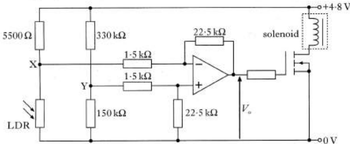
The potential at Y is 1.50 V. When the washing machine is filling with water, the narrow beam of light illuminates the LDR, the bridge is unbalanced and the potential at X is 1.28 V.
