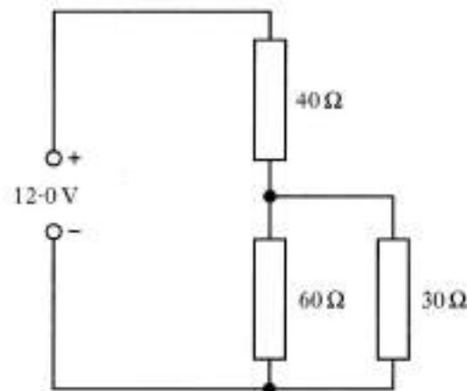
The p.d. across the  $30 \Omega$  resistor is
