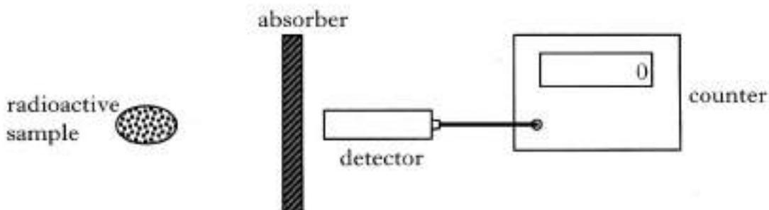
Different thicknesses of the absorber are placed in turn between the sample and the detector. For each thickness, the technician makes **repeated** measurements to obtain an average corrected count rate.
