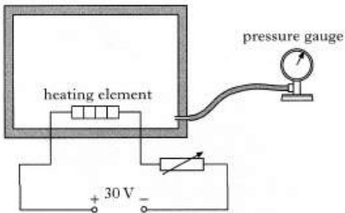
The heating element is used to raise the temperature of the gas.
