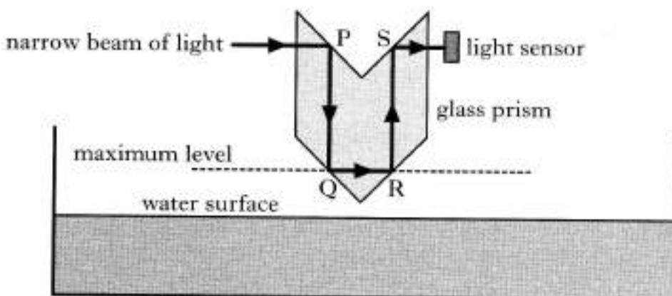
When the water in the machine is below the maximum level indicated in the diagram, the light sensor is illuminated by the narrow beam of light.
