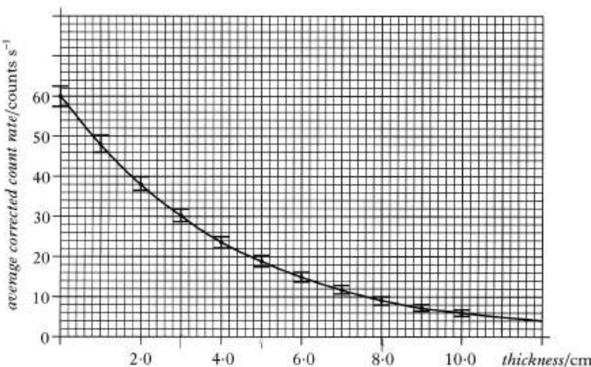
(i) Use the graph to calculate the half-value thickness of the absorber material for this radiation.
