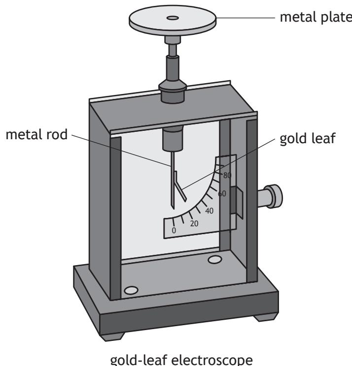
(a) Ultraviolet light is shone onto the negatively charged metal plate. The gold-leaf electroscope does not discharge. This indicates that photoelectrons are not ejected from the surface of the metal.
