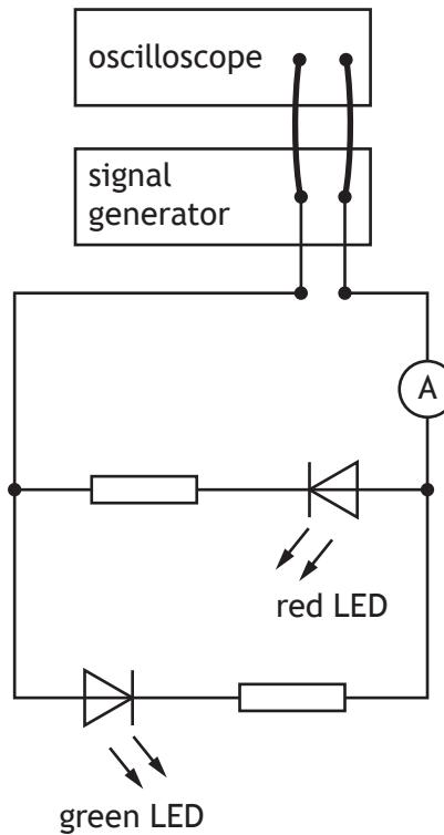
The output of the signal generator is displayed on the oscilloscope.
