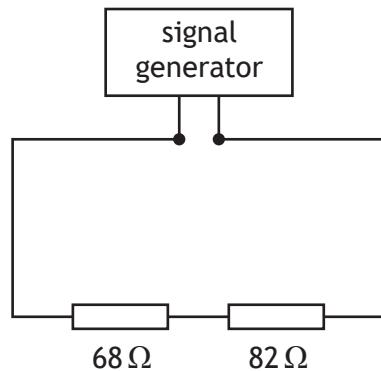
Determine the r.m.s. voltage across the  $82\ \Omega$  resistor.
