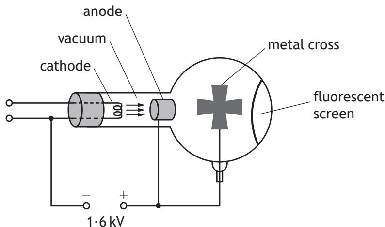
(a) Electrons are accelerated from rest between the cathode and the anode by a potential difference of 1.6 kV.
