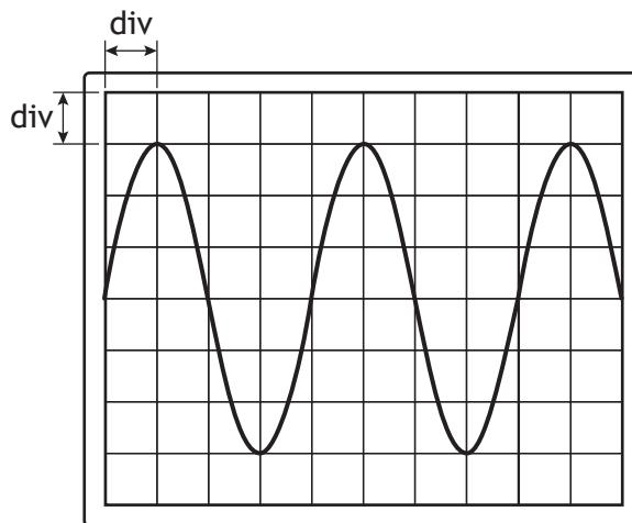
The Y-gain setting on the oscilloscope is 1.0 V/div.
