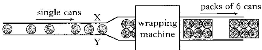
A light beam is set up across X-Y to send a signal to a counter. This signal operates the wrapping machine after six cans are detected.
