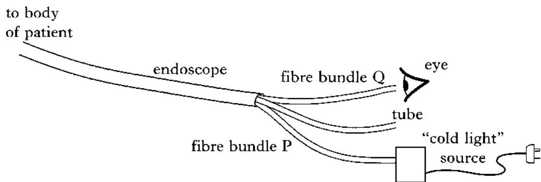
(a) (i) Explain the purpose of each of the two bundles of fibres in the endoscope.
