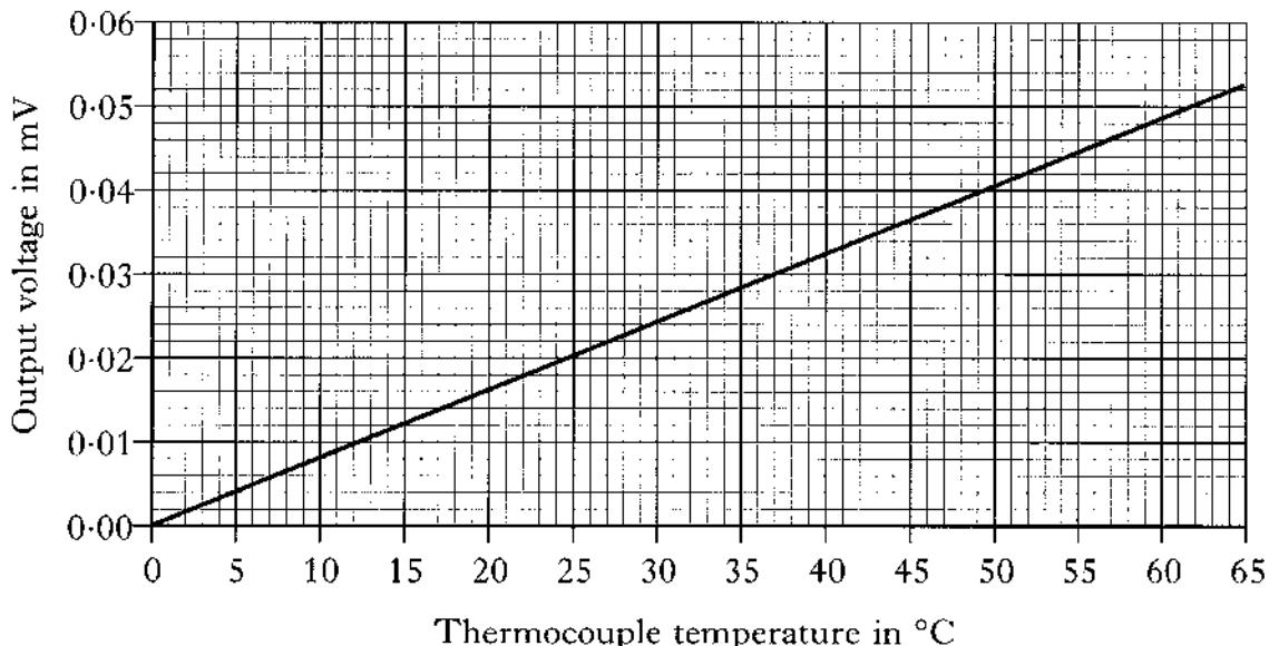
(i) What is the voltage produced by the thermocouple at 37 °C?
