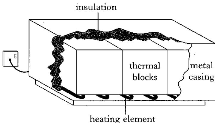
The heating element heats the thermal blocks during the night.
