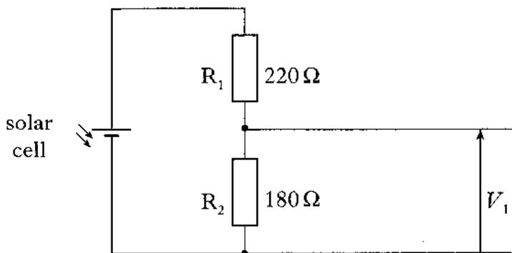
Calculate the voltage  $V_1$  when the solar cell is in a light level of 500 lux.
