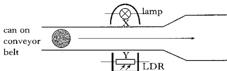
(a) The circuit shown produces the input signal for the counter.
