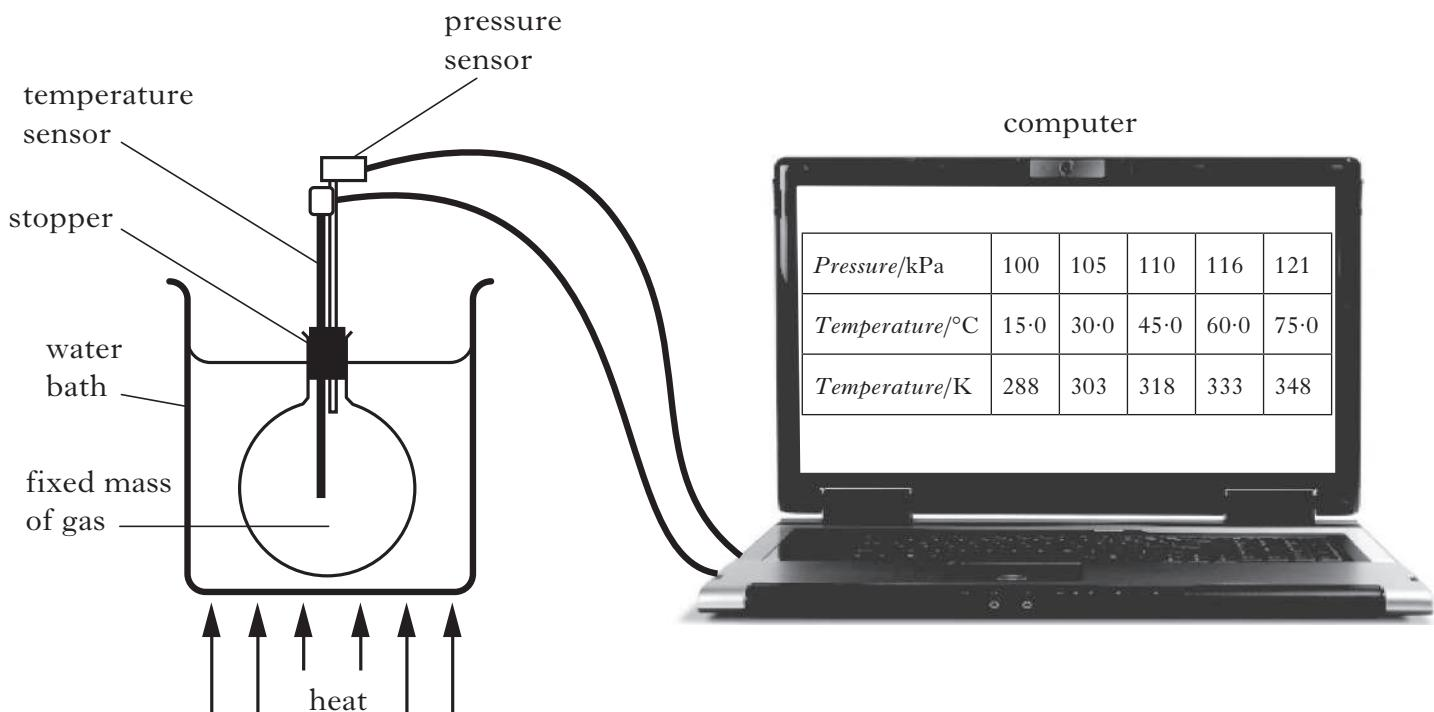
The pressure and temperature of the gas are recorded using sensors connected to a computer. The gas is heated slowly in the water bath and a series of readings is taken.
