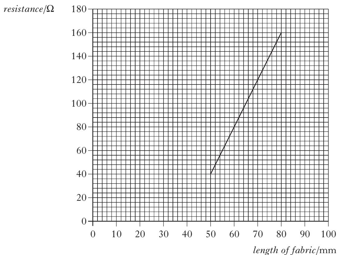
A sample of the fabric of unstretched length 50 mm is connected in a Wheatstone bridge circuit.
