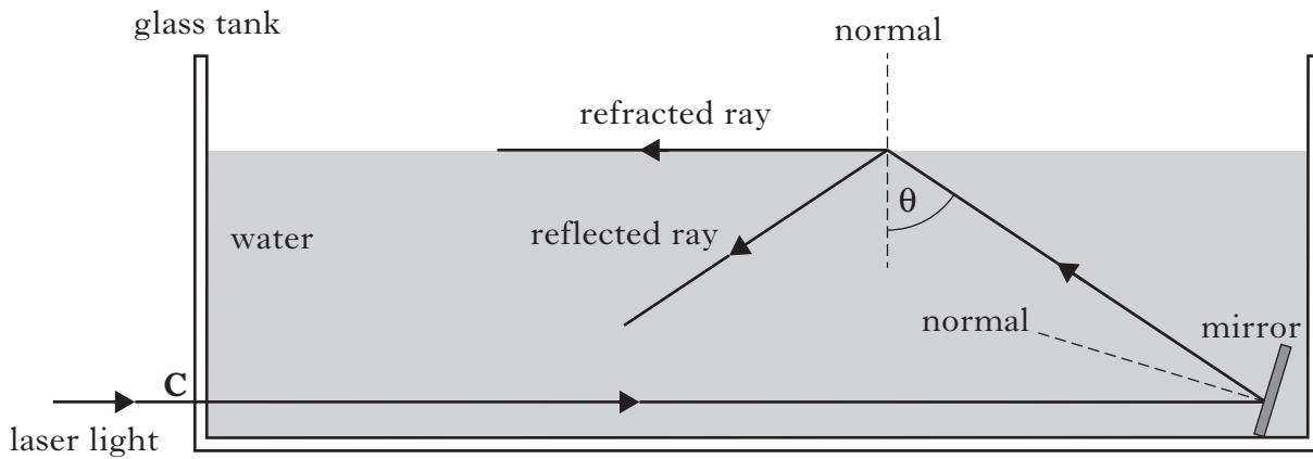
(i) State why the value of  $\theta$  is equal to the critical angle for this laser light in water. 1
