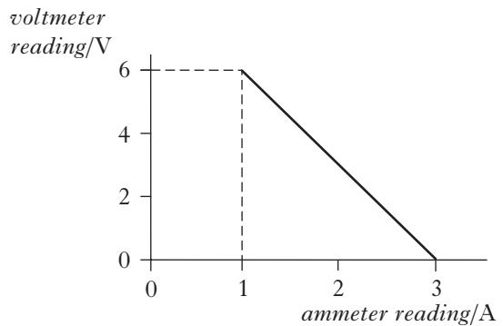
Which row in the table shows the values for the e.m.f. and internal resistance of the battery in the circuit?
