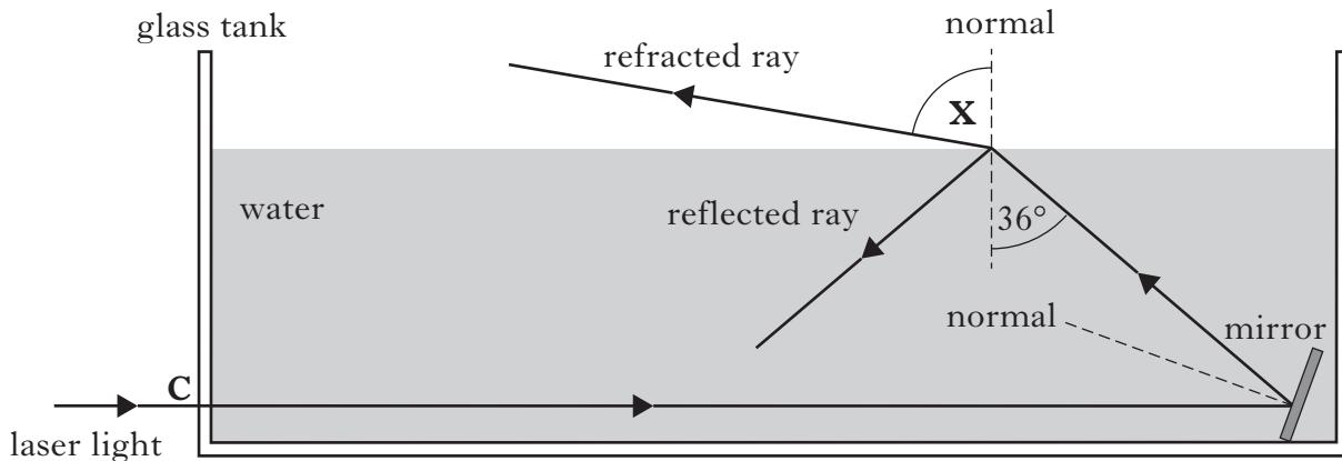
The refractive index of water for this laser light is 1.33.
