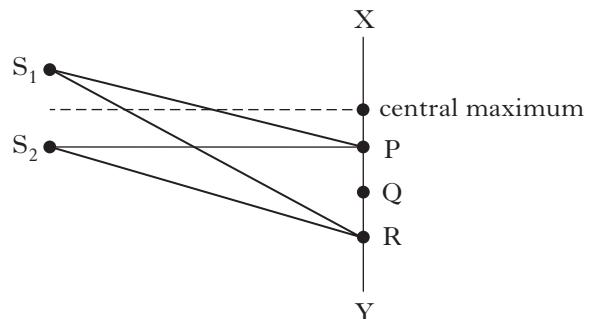
The first order maximum occurs at P, where  $S_1P = 200 \text{ mm}$  and  $S_2P = 180 \text{ mm}$ .
