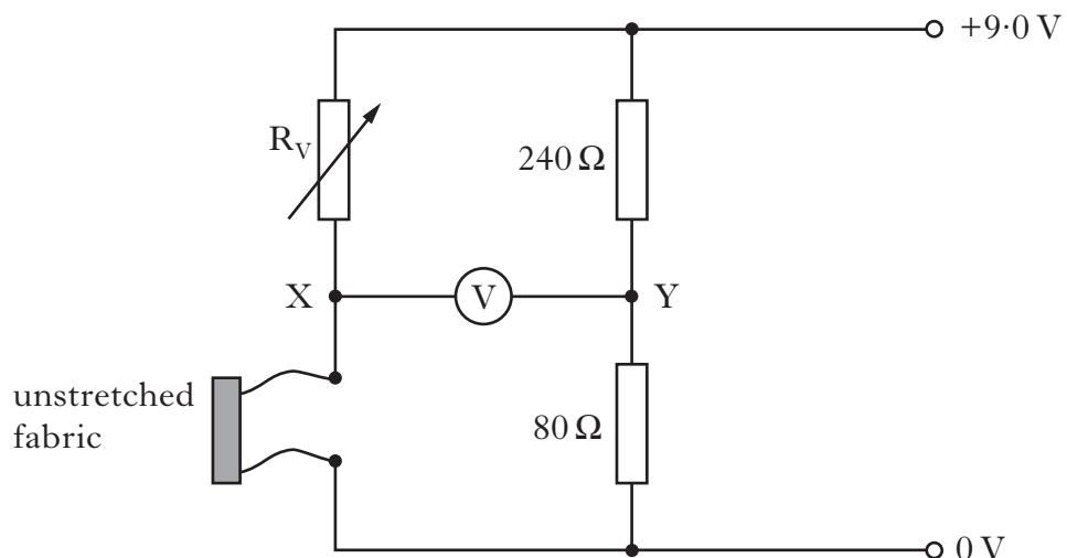
(a) The variable resistor  $R_V$  is adjusted until the bridge is balanced.
