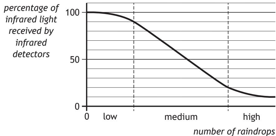
The percentage of infrared light received by the infrared detectors from the LEDs controls the frequency with which the windscreen wipers move back and forth.
