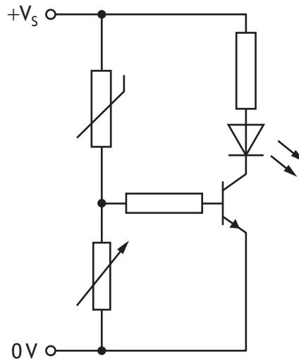
The variable resistor is adjusted until the LED switches off.
