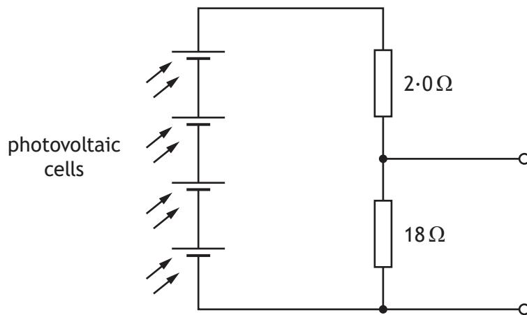
In direct sunlight the photovoltaic cells produce a combined voltage of 4.0 V.
