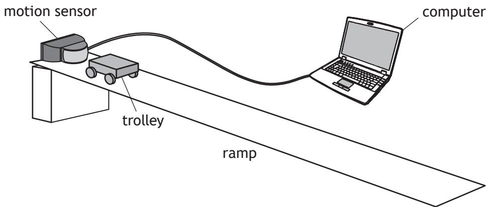
The student releases the trolley. The computer displays the velocity-time graph for the motion of the trolley as it rolls down the ramp, as shown.
