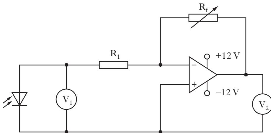
(i) In which mode is the photodiode being used? 1
