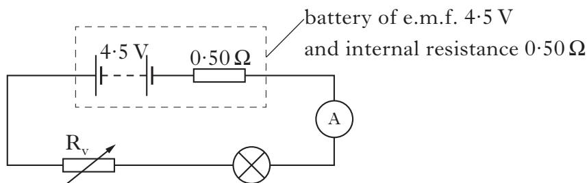
(a) The resistance of variable resistor  $R_v$  is set to  $2.5\ \Omega$ . The reading on the ammeter is  $0.30\ A$ .
