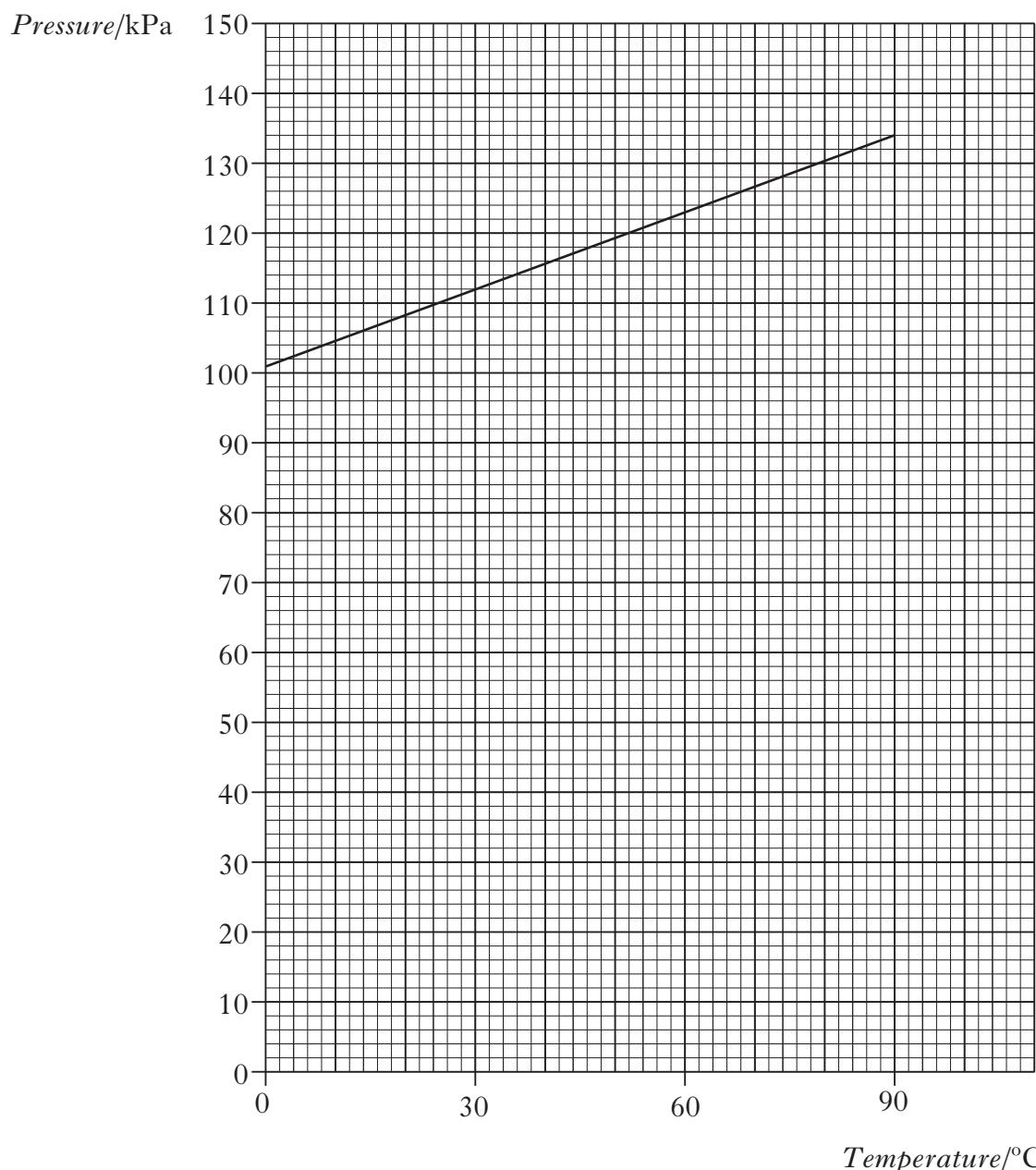
(a) The student deduces that the pressure is **not** directly proportional to the temperature of the gas in degrees celsius.
