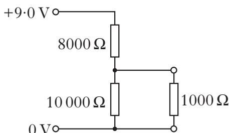
State which student's design achieves a potential difference closer to 5.0 V across the 1000 Ω load resistor.
