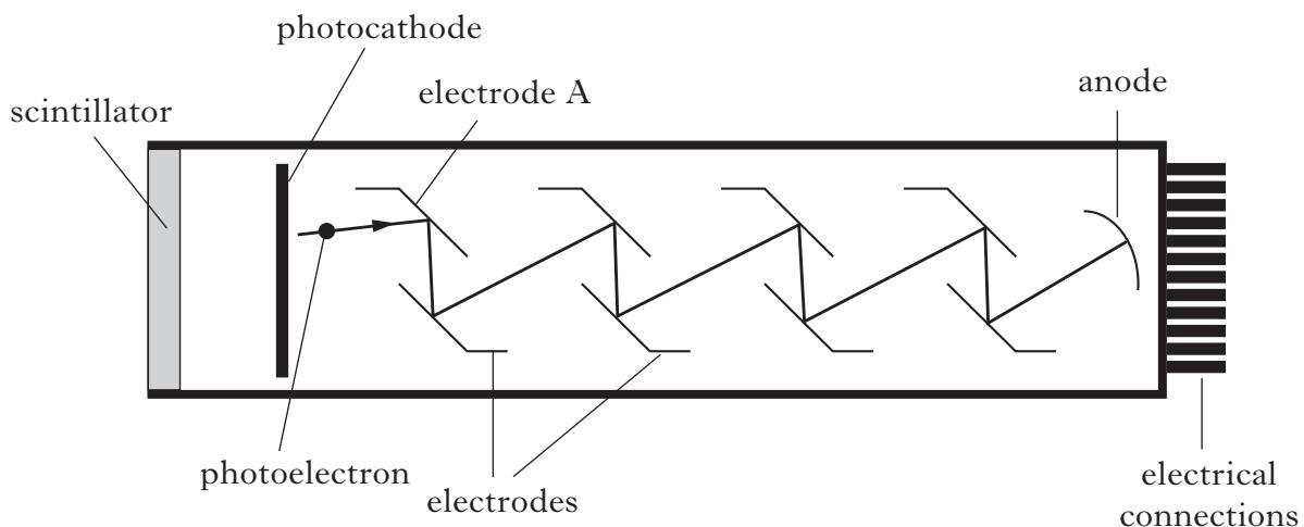
A particular photoelectron is released from the photocathode with a kinetic energy of  $1.36 \times 10^{-19} \text{ J}$ . It is then accelerated by a potential difference of 120 V between the photocathode and electrode A.
