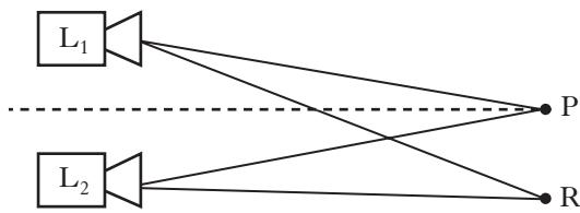
At position P, which is the same distance from both loudspeakers, there is a maximum.
