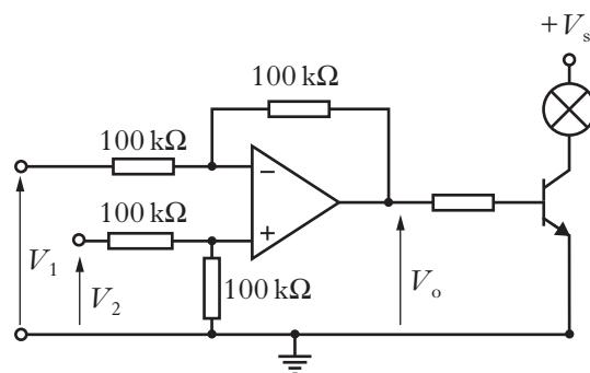
The transistor switches on when  $V_o = 0.7$  V.
