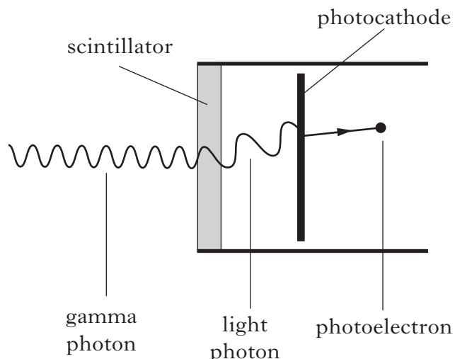
The work function of the photocathode is  $3.20 \times 10^{-19} \text{ J}$ .
