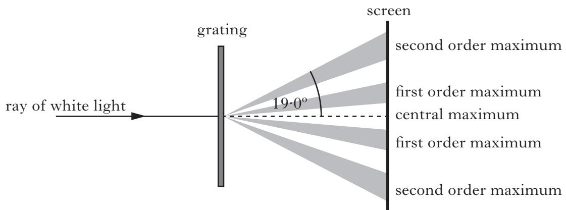
The angle between the central maximum and the second order maximum for red light is  $19.0^\circ$ .
