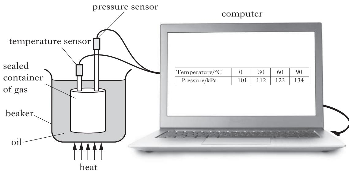
A sealed container of gas is submerged in a beaker of oil.
