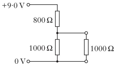
Calculate the potential difference across the load resistor. 2
