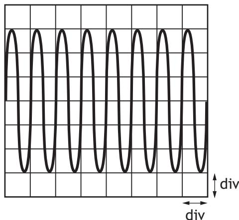
The timebase control of the oscilloscope is set at 2 ms/div.
