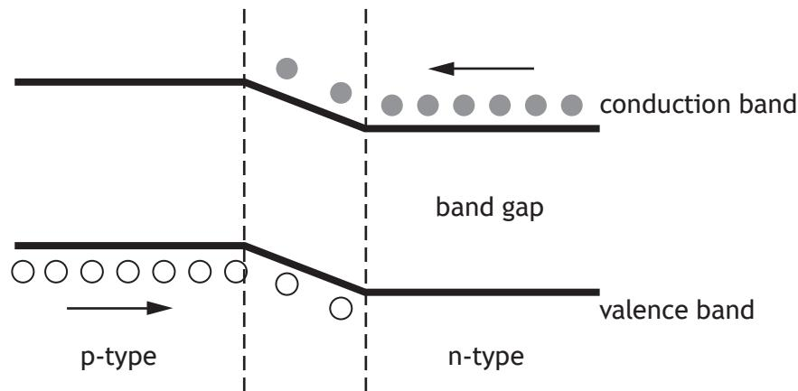
(i) A voltage is applied across an LED so that it is forward biased and emits light.
