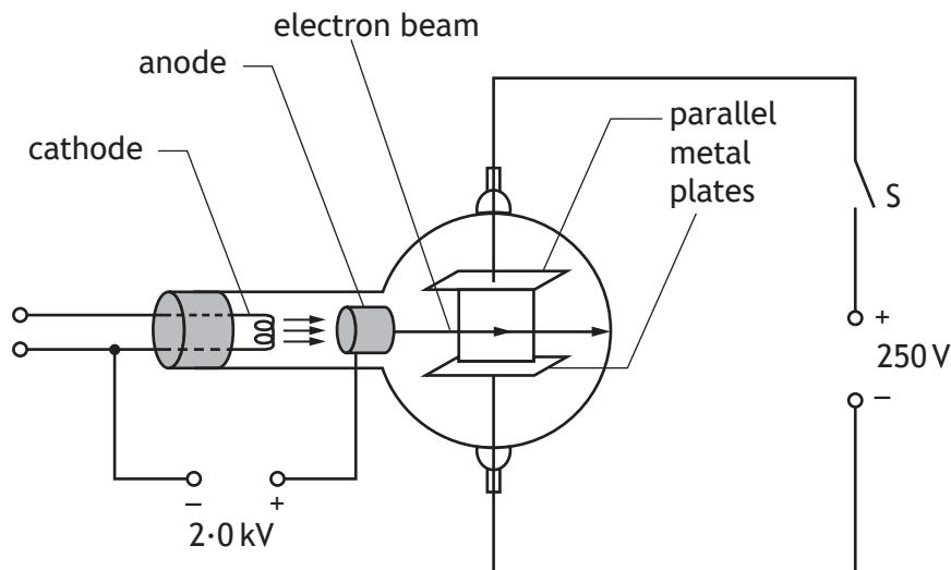
(a) Electrons are accelerated from rest between the cathode and the anode by a potential difference of 2.0 kV.
