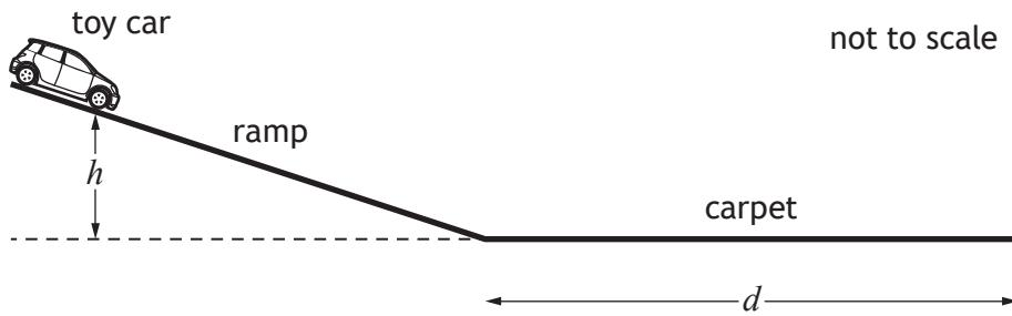
The toy car is released from rest, from a height  $h$ . It then travels down the ramp and along the carpet before coming to rest. The student measures the distance  $d$  that the car travels along the carpet.
