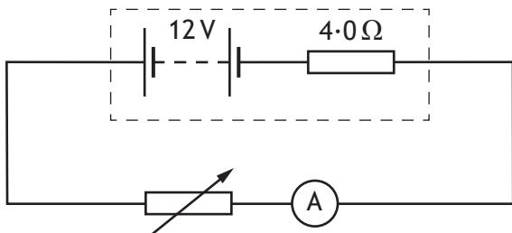
The resistance of the variable resistor is increased and corresponding readings on the ammeter are recorded.
