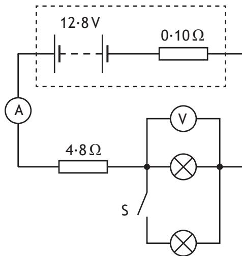
(a) Switch S is open. The reading on the ammeter is 1.80 A.
