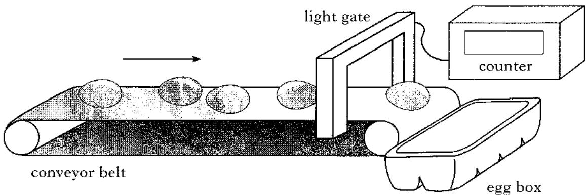
(a) The light gate consists of a light source and detector.
