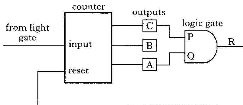
The input to the counter goes to logic 1 every time an egg passes through the light gate. When the reset to the counter goes to logic 1, the outputs go to zero.
