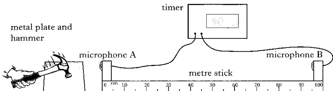
Striking the metal plate with the hammer produces a sound. Timing starts when the sound reaches microphone A, and stops when the same sound reaches microphone B.
