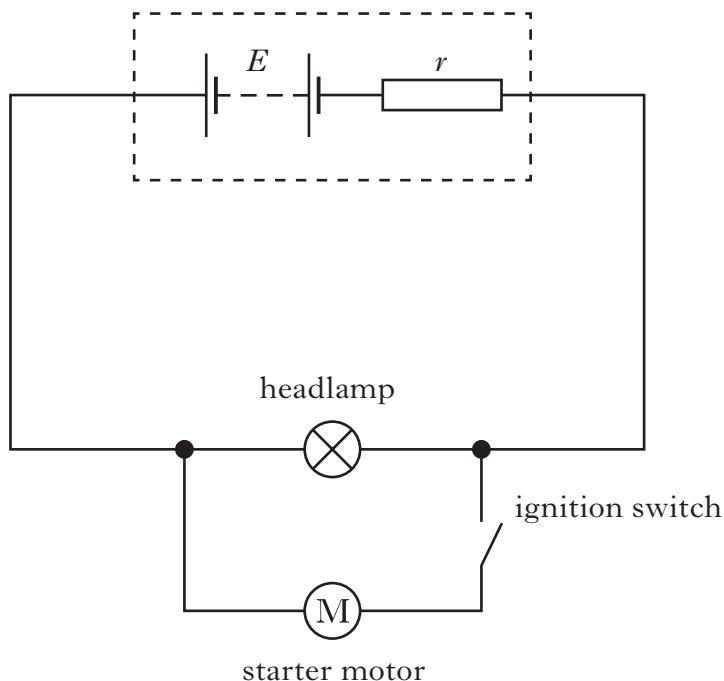
The technician notices that the headlamp becomes dimmer when the ignition switch is closed and the starter motor operates.
