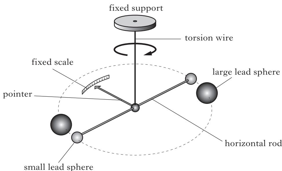
The torsion wire twists by one degree when each small lead sphere experiences a force of  $1.56 \times 10^{-9}$  N.
