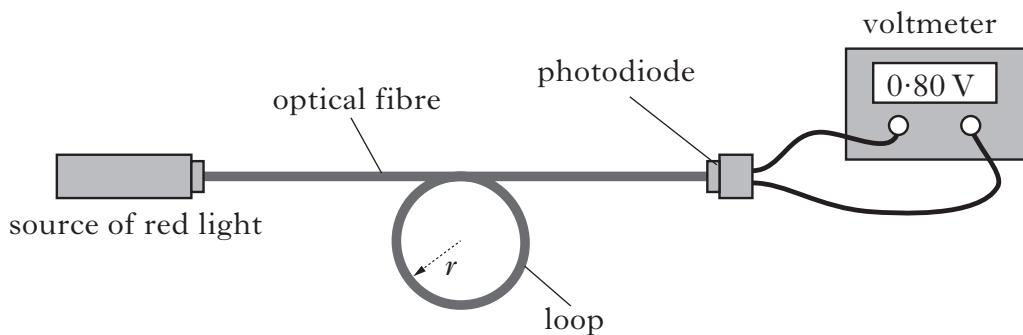
The photodiode produces a voltage proportional to the irradiance of light incident on it.
