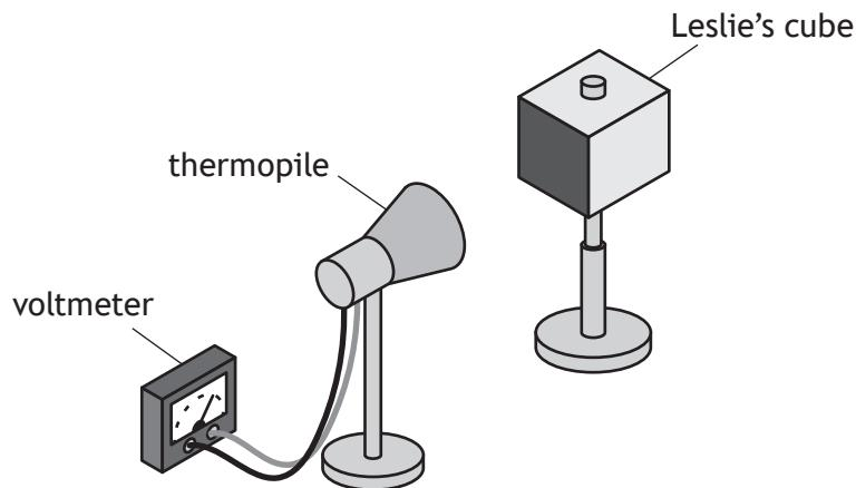
The student fills the cube with hot water and measures the amount of infrared radiation at different distances from the cube, using the thermopile.
