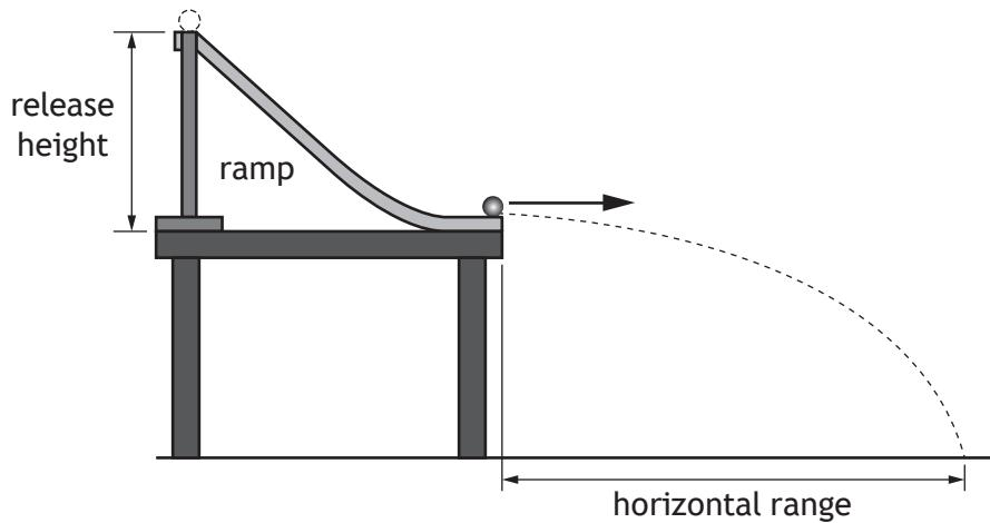
(a) The student releases a marble from different heights on the ramp and measures the horizontal range.
