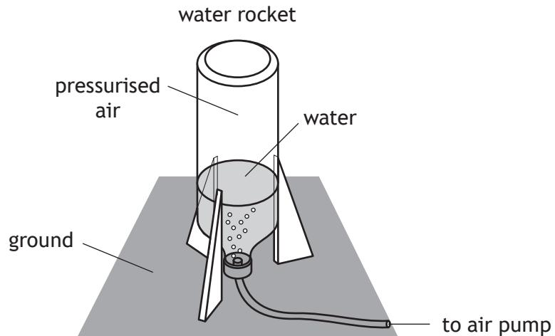
Air is pumped into the rocket until the pressure of the air inside is large enough for the water rocket to launch upwards.
