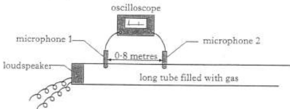
A pulse of sound from the loudspeaker is directed along the tube. The sound detected by each microphone produces a peak on the oscilloscope screen.
