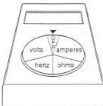
What is the correct setting of the dial when the meter is used to measure frequency?
