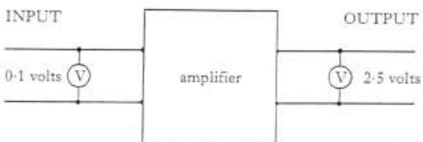
(i) Calculate the voltage gain of this amplifier.
