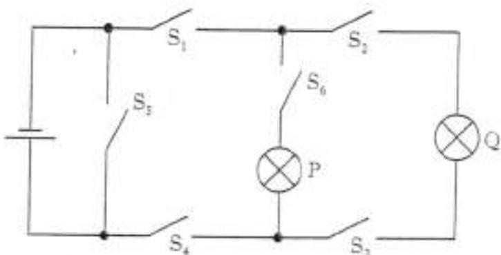
(i) Which switches should be closed so that **only** lamp P lights?
