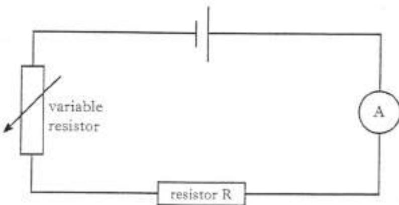
(i) On the diagram above, add a voltmeter to show how the voltage across resistor R could be measured.
