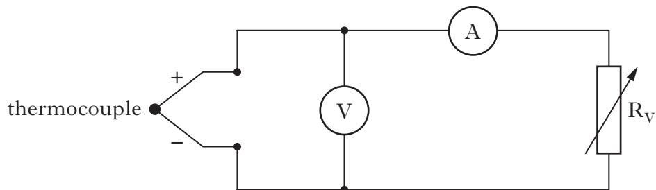
Readings of current and potential difference (p.d.) are recorded for different settings of the variable resistor  $R_V$ .
