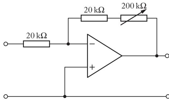
In this circuit, adjustment of the resistance of the variable resistor from zero to  $200\text{ k}\Omega$  allows the voltage gain to be altered over the range
