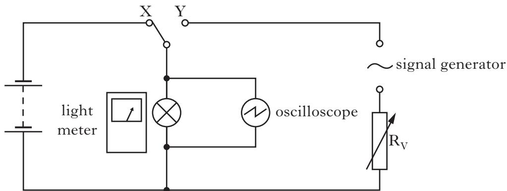
The switch is connected to X and the voltage across the lamp is 2.30 V. The reading on the light meter is recorded.
