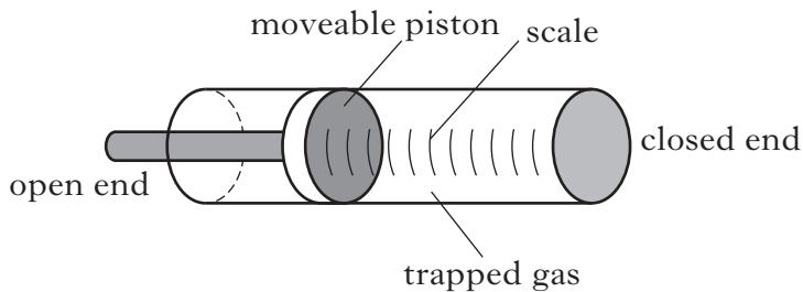
At sea level, the atmospheric pressure is  $1.01 \times 10^5 \text{ Pa}$  and the trapped gas exerts a force of  $262 \text{ N}$  on the piston.
