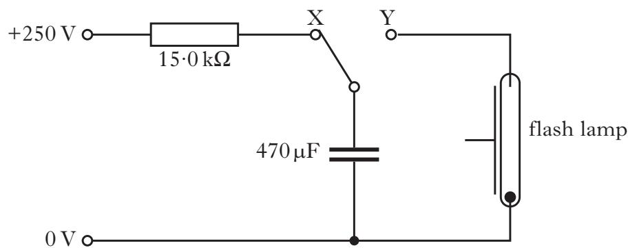
(a) The capacitor is now charged by connecting the switch to X.
