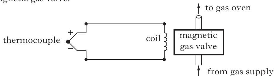
When the current in the coil is less than  $2.5\text{ A}$ , the gas valve is closed.
