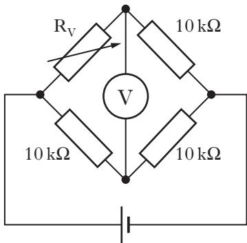
The reading on the voltmeter is zero.
