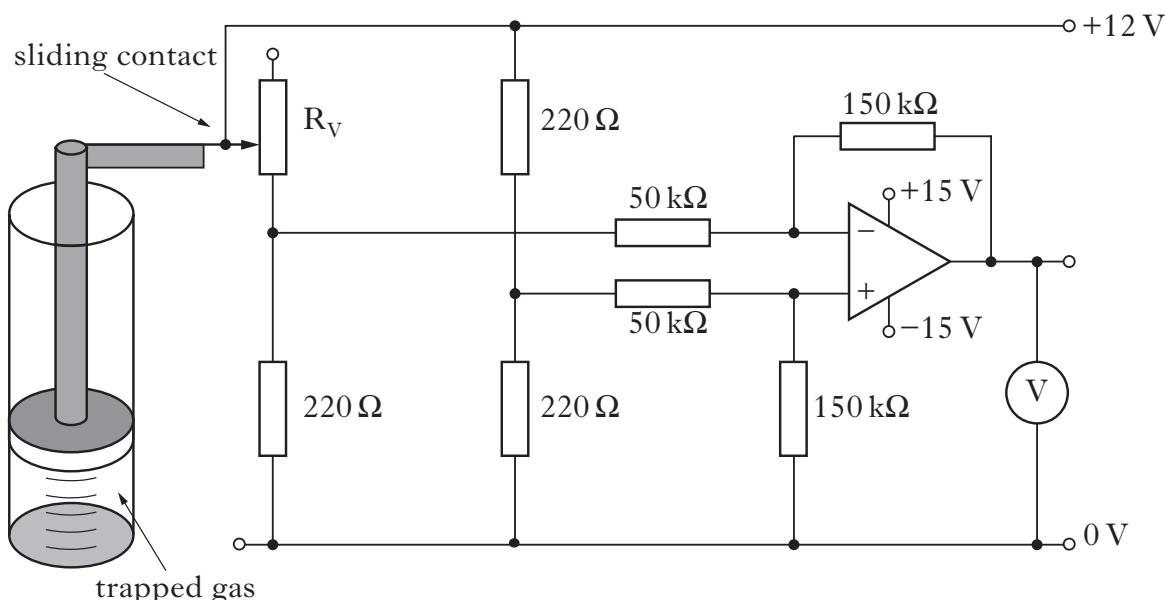
The resistance of  $R_V$  decreases as the depth of the mini-submarine increases.
