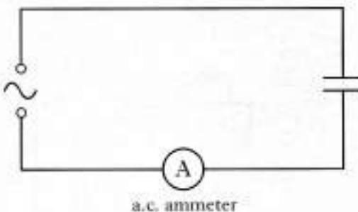
The alternating supply has a constant peak voltage but its frequency can be varied.
