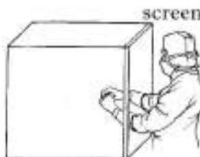
(a) The screen must be sufficiently thick to reduce the radiation to an acceptable level.
