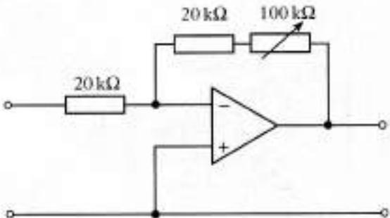
The variable resistor can be adjusted from zero to  $100\text{ k}\Omega$ . This allows the voltage gain to be altered over the range
