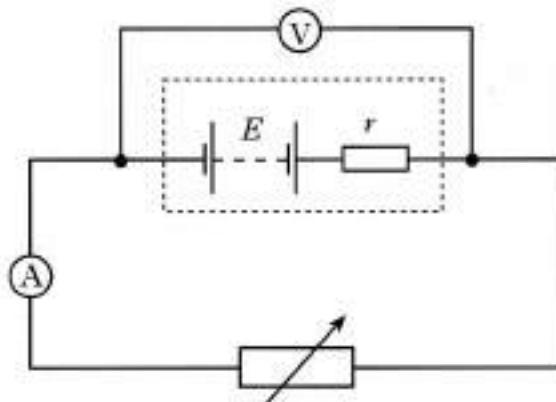
Readings from the voltmeter and ammeter are used to plot the following graph.
