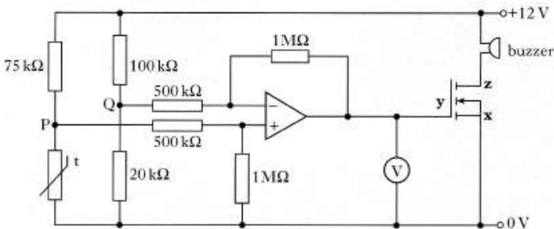
(a) What names are given to the terminals labelled **x**, **y** and **z** on the symbol for the MOSFET?
