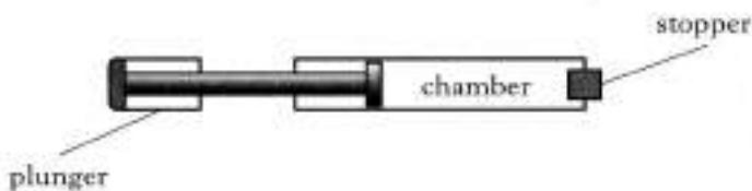
The plunger is now pushed in slowly causing the air in the chamber to be compressed. As a result of this the pressure of the trapped air increases.
