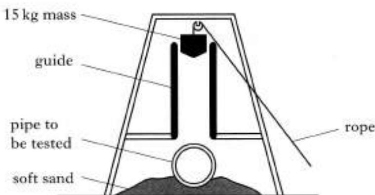
When the rope is released, the 15 kg mass is dropped and falls freely through a distance of 2.0 m on to the pipe.
