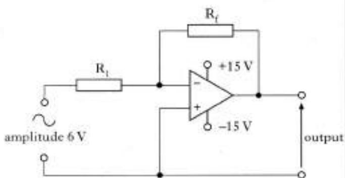
Which values for resistors  $R_1$  and  $R_f$  will produce an approximate square wave output?
