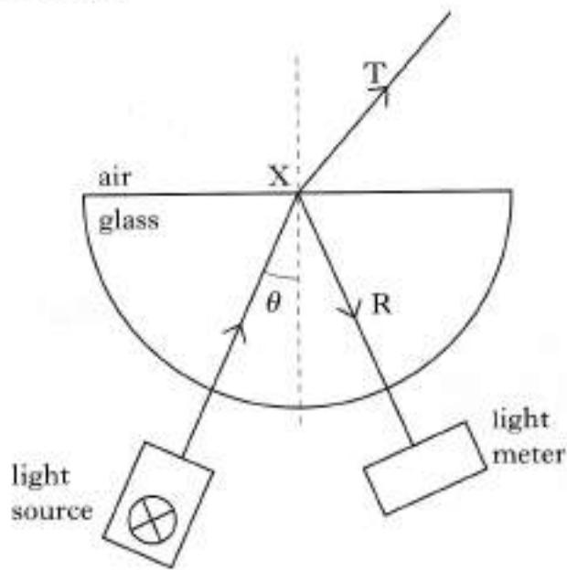
The student uses a light meter to measure the intensity of ray R as angle  $\theta$  is changed.
