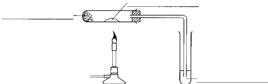
(a) Label the diagram of the apparatus used to crack liquid paraffin.
