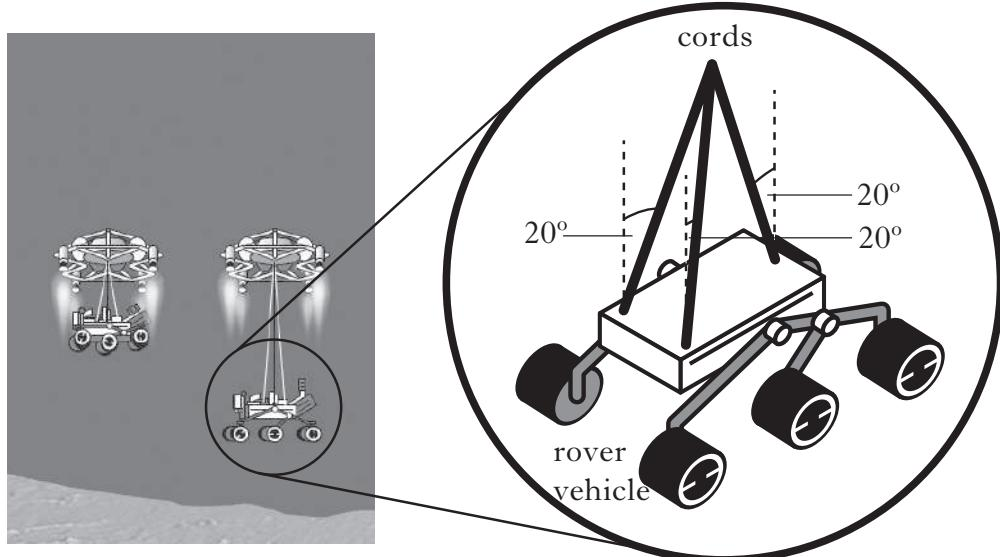
The rover vehicle has a weight of  $1380 \text{ N}$ .
